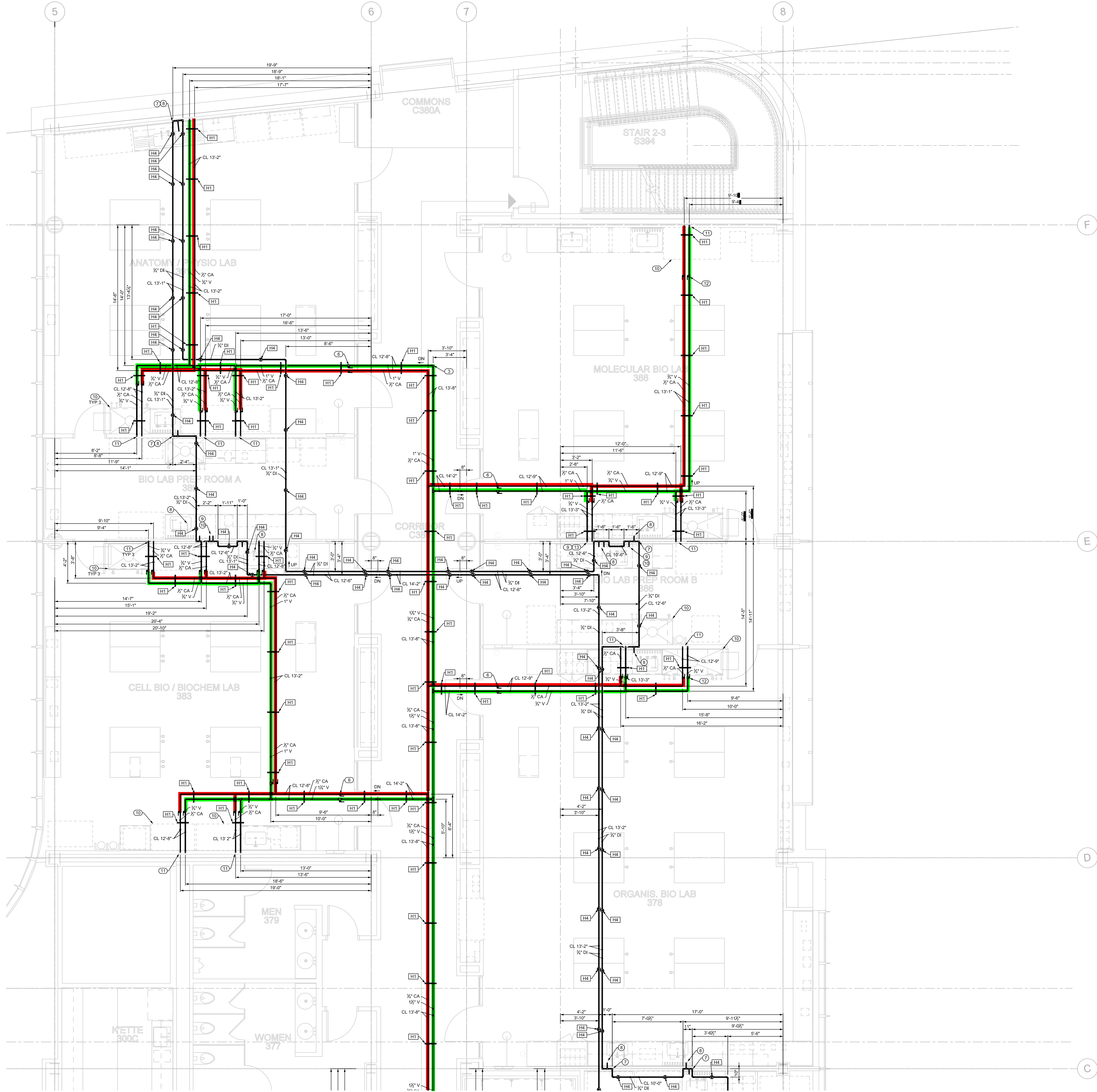
1 PARTIAL LEVEL 3 - LAB GAS PIPING PLAN SCALE: 1/4"=1'-0"
